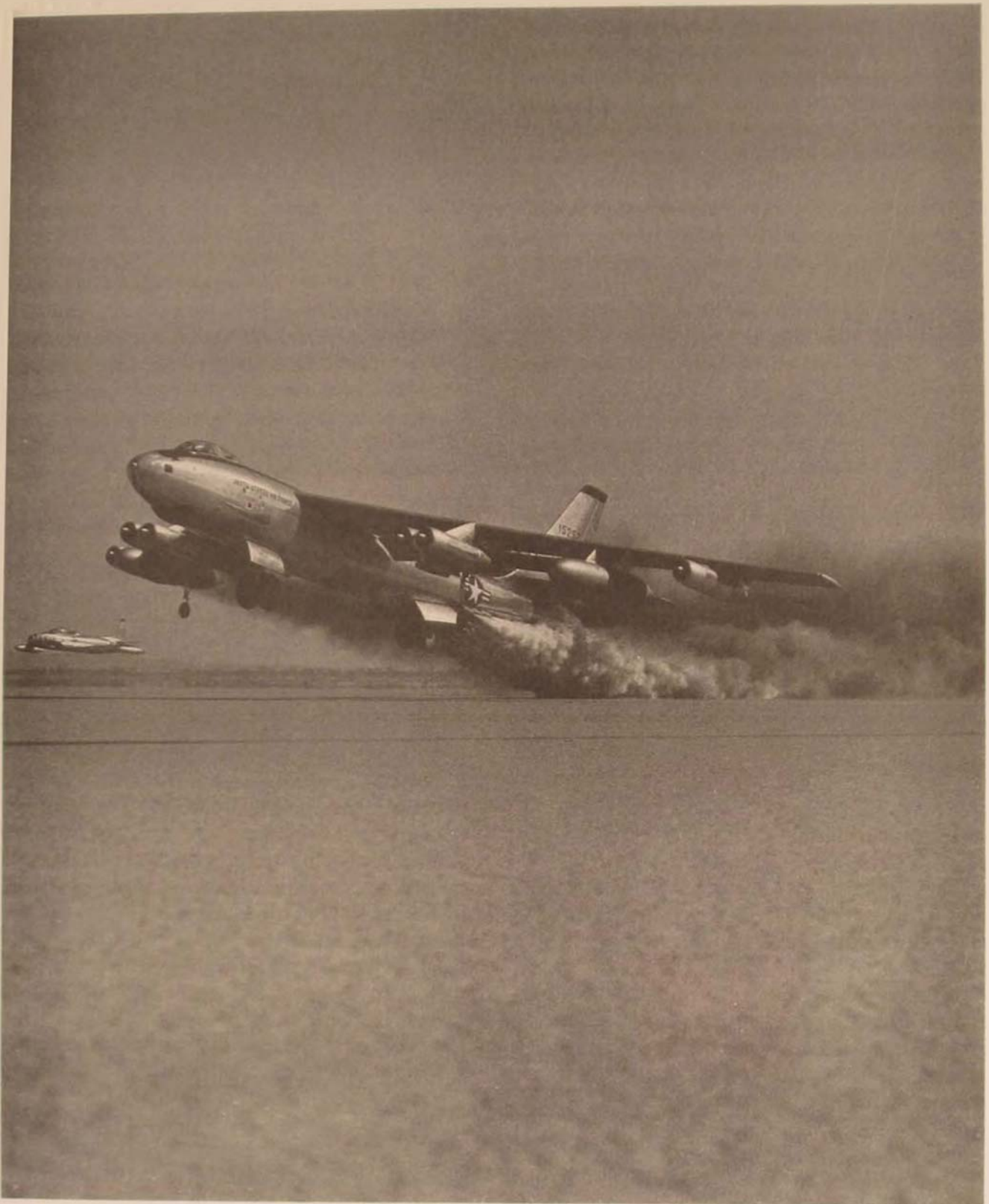
The first in a new breed—a B-47 with jet-assisted takeoff (JATO) undergoes testing at Edwards AFB, California.
